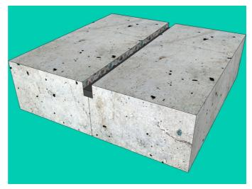
keep firm hand pressure on the repair area until the plug has hardened. Insure that Crystal Stop does not exceed 1/2 of the channel height.
