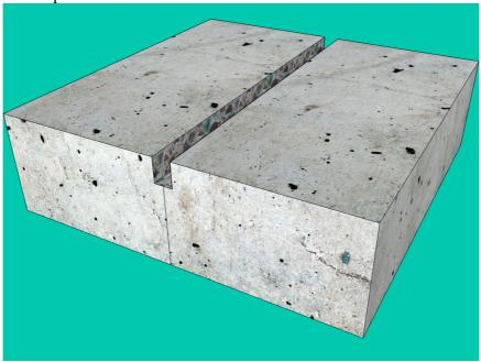
Insure that all cracks are channeled at least 10 cm beyond the visible end of the crack. In areas in which structural reinforcing steel does not allow 3.5 cm consistently, chip or chisel or route the concrete on both sides of the steel to the appropriate depth and clear the area over the steel to whatever depth is allow by the placement of the steel.
